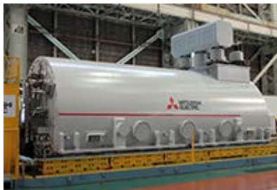
870MVA verified generator
