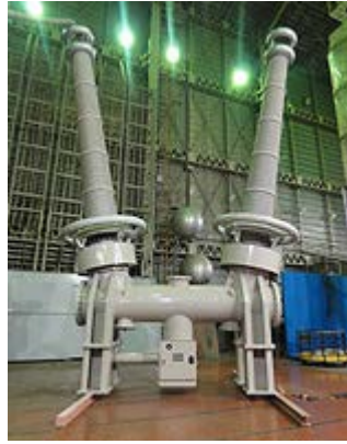
Gas circuit breaker
